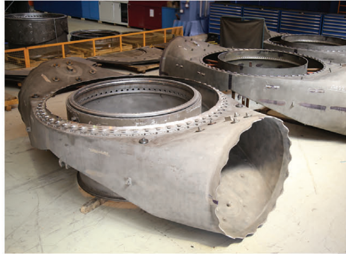
Hot gas path of gas turbine equipment
