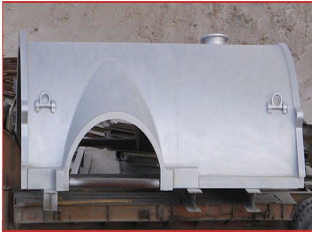
Gas turbine casing
